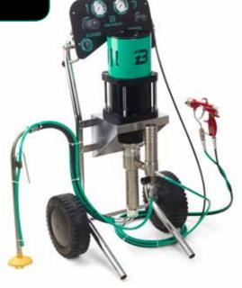
Piston pneumatic air-assisted airless pump for medium pressure professional paint spraying, suitable for the wood and metal sectors. Available in the airless model.
