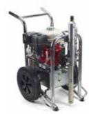
CODE **DESCRIPTION** TKH21G MIURA 21000 Hydraulic airless piston pump with gas engine C/Trolley - Inline filter - Manometer - HP hose 10m - RST2 spray gun - FM6 tip guard - Reversible FM6 tip -Direct suction
